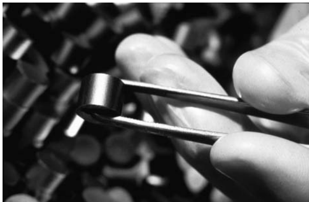
FIGURE 9.3 Single fuel pellet prior to insertion into a fuel rod.
