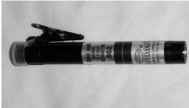
FIGURE 19.16 Pocket dosimeter. (Courtesy of Paul Frame.)
