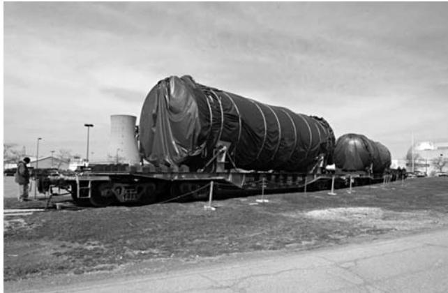
FIGURE 13.6 Large power plant components in an SCO-1 packaging (MHF P: Pictures Femi II MSRs ar FERMI MSR 99).
