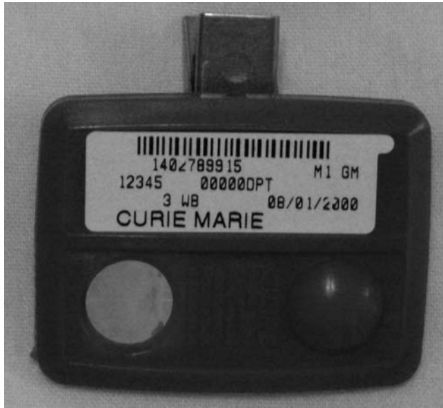
FIGURE 19.14 Film badge. (Courtesy of MP Dosimetry.)
